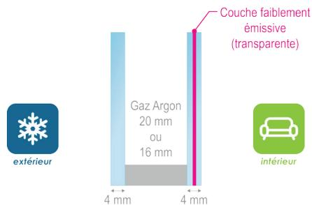
$U_g = 1.1 \text{ W}/(\text{m}^2.\text{K})$
