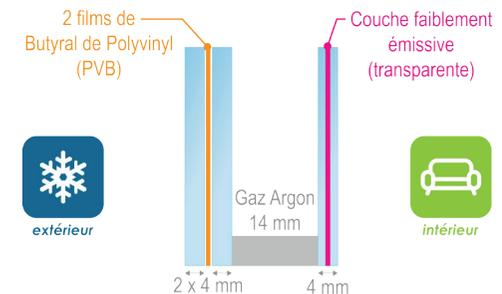
$U_g = 1.1 \text{ W}/(\text{m}^2.\text{K})$
