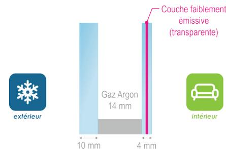
$U_g = 1.1 \text{ W}/(\text{m}^2.\text{K})$
